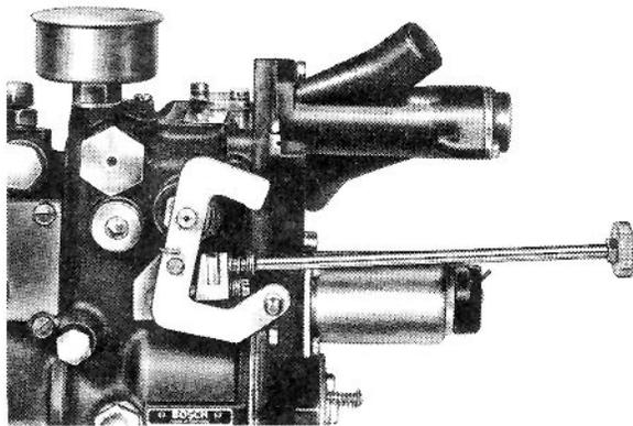
The principle advantage of the specially made tool is that the throttle valve angle does not change if acceleration is necessary during the measurement, due to traffic conditions.
