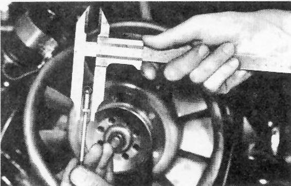
**“Basic adjustment”** of throttle valve push rods.
