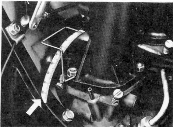
The arrow indicates the place where the right protractor can touch on the 2.4 and 2.7 liter engines. Reshape the protractor.
