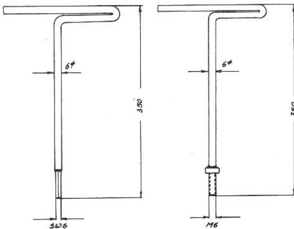
**T grip spanner with end section for socket head screws** (left-hand illustration)
