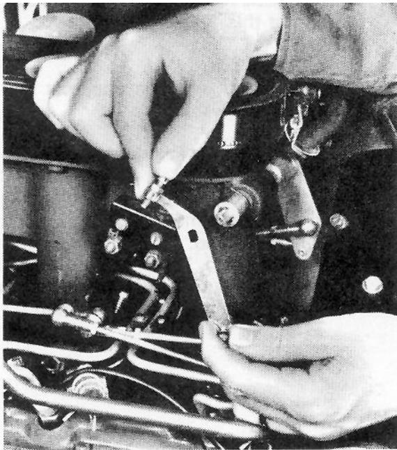
2. Re-engage the correctly adjusted connecting rod. The measurement for the push rods from the cross shaft to the throttle valve housing is thus established.
